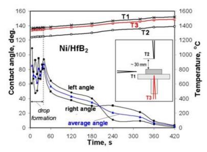
Fig. 1. Wetting behavior of the Ni/HfB<sub>2</sub> couple during contact heating to 1450°C with the corresponding temperature profile recorded by three thermocouples (T1, T2 and T3)
