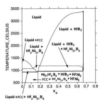
Fig. 2. Calculated isopleth along the Ni-HfB<sub>2</sub> join [17], given by the equation:  $X_B - 2 \cdot X_{Hf} = 0$ , where  $0 < X_{Hf} < 0.333$  and the sum of the mole fractions of  $(X_B + X_{Hf} + X_{Ni}) = 1$
