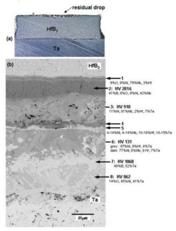
Fig. 3. OM image of cross-sectioned Ta/Ni-B/HfB<sub>2</sub> joint structure (a) and its SEM/EDS/microhardness analysis (b)
