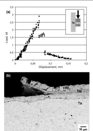
Fig. 4. Shear behavior of Ta/Ni-B/HfB<sub>2</sub> joint (a) and cross-section of the joint after shear test (b) showing failure in the HfB<sub>2</sub> substrate and cracking at the interface between Nb layer and the newly formed transition multilayer region
