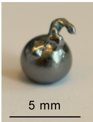
Fig. 1. An example of Si-13.5B alloy sample fabricated by crucible less electric arc melting method, at Leibnitz Institute for Solid State and Materials Research (Dresden, Germany)
