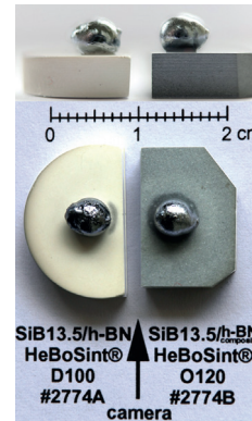
Fig. 5. A macroview of the couple A: Si-13.5B/h-BN and couple B: Si-13.5B/(h-BN + SiC + ZrO 2 ) composite after the sessile drop test performed by “2 in 1” testing procedure
