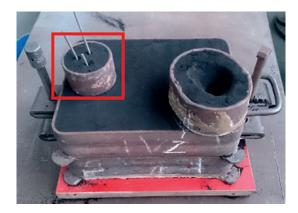
Fig. 2. Casting mould showing marked place where samples were taken for the determination of gas content
