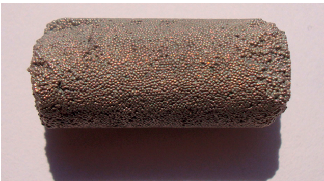
Fig. 3. Compact body of ordered hollow ceramic spheres connected with nickel
