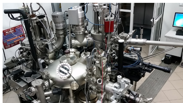
Fig. 1. Experimental complex for high-temperature studies of interaction between liquid metals and alloys with refractory materials [23]
