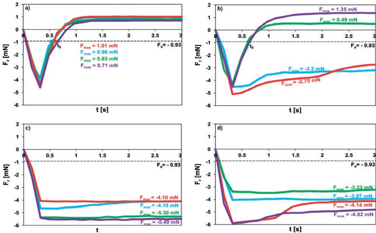
Fig. 2. Wetting balance curves recorded during the solderability tests of PCBs with OSP finish by SAC305 (4 samples for each kind of PCB finish were done): a) in delivery state (reference), b) after mechanical damage, c) oxidized in air (260°C, 1 h), d) after oxidation and mechanical damage
