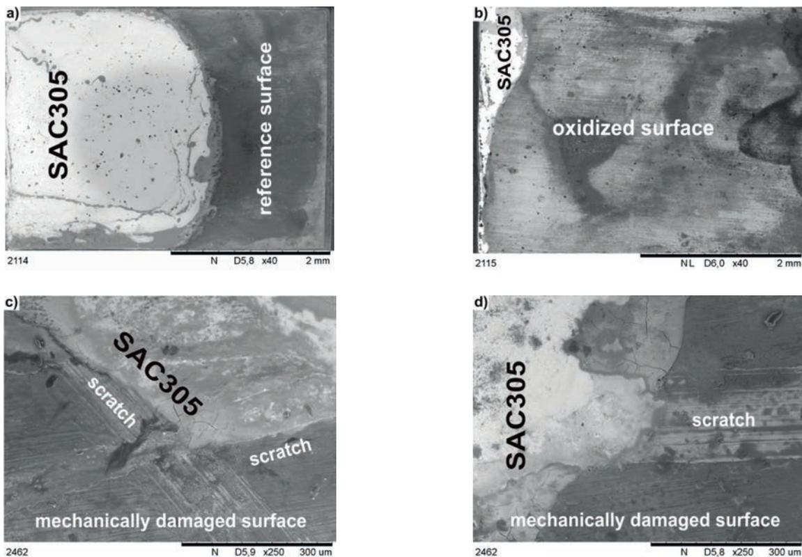
Fig. 5. SEM images: a) in delivery state (reference), mag.  $\times 40$ , b) after oxidation in air ( $260^\circ\text{C}$ , 1 h), mag.  $\times 40$ , c) after mechanical damage (scratch parallel to solder), mag.  $\times 250$ , d) after mechanical damage (scratch perpendicular to solder), mag.  $\times 250$
