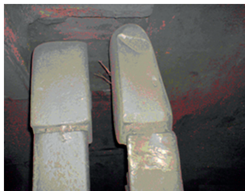
Fig. 1. Worn-out hammers for crushing of lignite made of GE 300 steel
