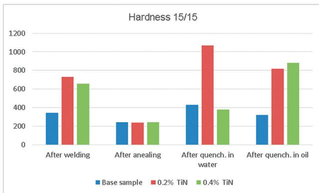
Fig. 10. Hardness after heat treatment
