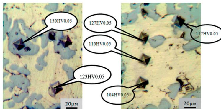
Fig. 4. Microstructure  $\times 500$  before etching of the obtained MMC, by measured Vickers microhardness in the area of the matrix and a reinforcement phase
