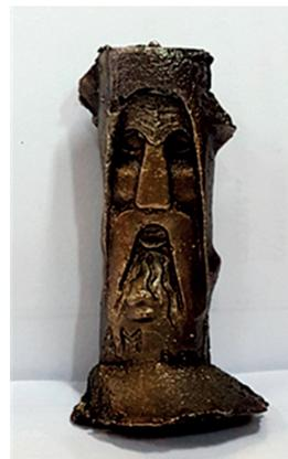
Fig. 2. Picture of the obtained complex relief MMC with copper alloy (CuZn38Pb2) matrix and Fe reinforcing phase
