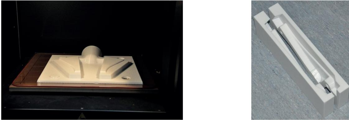
Fig. 10. Printed plate pattern and core box
