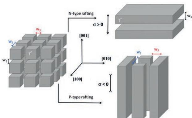
Fig. 1. Scheme of N- and P-type rafting in superalloys strengthened by cubic-shaped  $\gamma'$  precipitates [5]
