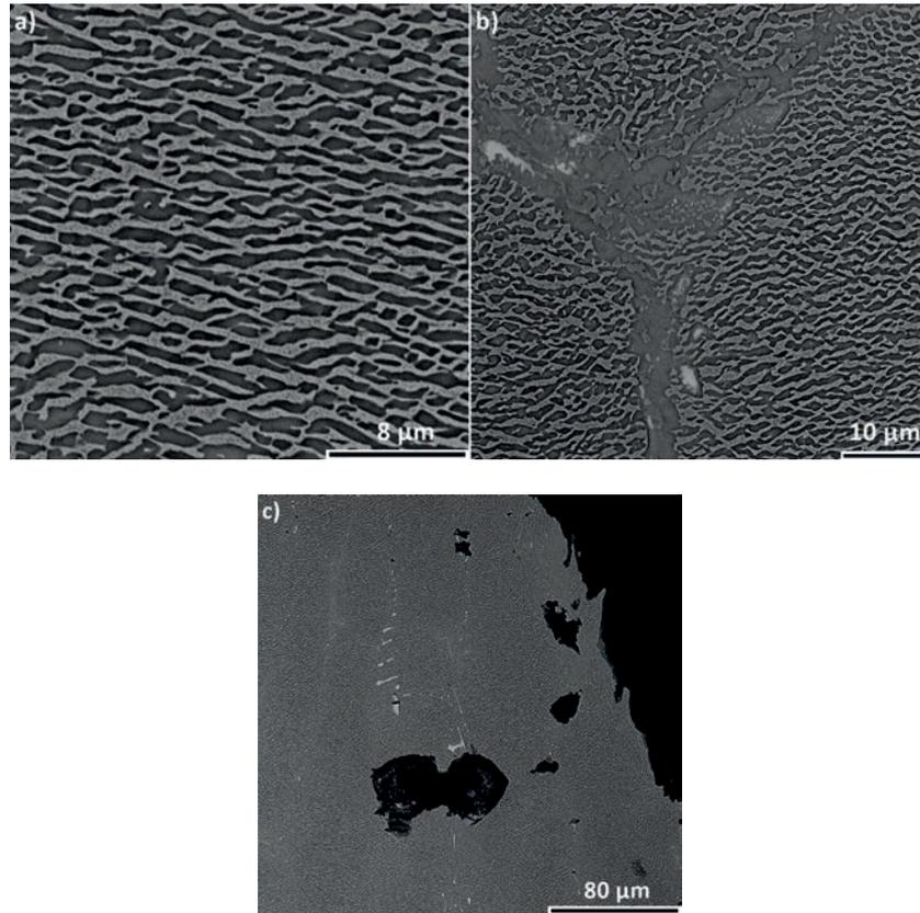
Fig. 7. Microstructural changes after creep: a) dendrite core, b) interdendritic space, c) voids inside the material
