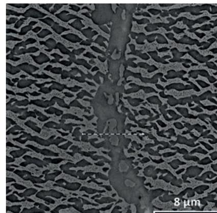
Fig. 8. Location of EDS line scan across grain boundary
