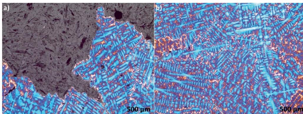
Fig. 6. Microstructure of crept sample: a) fracture, b) small local voids along grain boundaries
